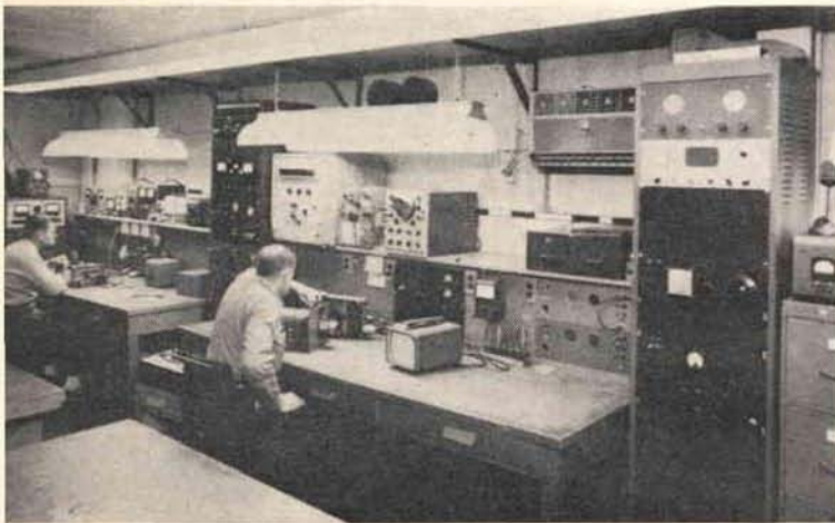
Fig. 7. This is just one corner of the electronic maintenance shop. A closed-circuit TV camera is being repaired. Equipment includes scopes, modulation monitors, deviation meters, frequency meters, wattmeters, and a WWV receiver.
