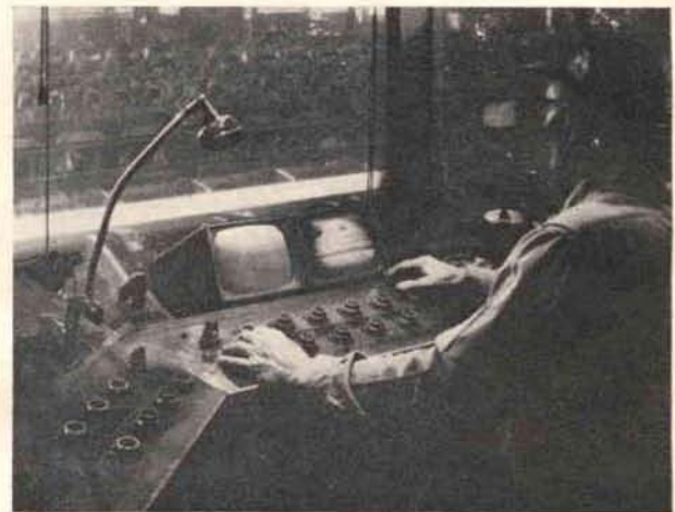
Fig. 8. An operator in a control pulpit, who makes certain that steel tubes are in the right position, observes the course of this steel on two separate monitor TV sets. He keeps an eye on two conditioning furnaces at the same time.
