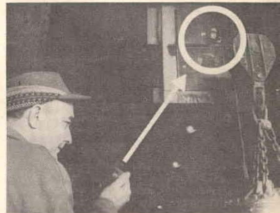
Fig. 6. A floor man guides the operator of the cab in an overhead crane in the steel mill through carrier-current radio. Hand signals are taboo.
